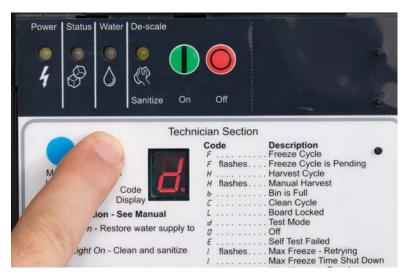
The control can be put into a Test Cycle, where it switches all the loads on and off in a logical sequence. This allows the technician to confirm controller operation of all parts.
