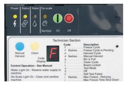
At the beginning of any restart or the first cycle after start up, the controller will display a blinking F.
