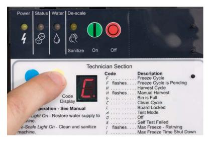
After 6 months of power up time, the De-Scale & Sanitize light will be switched On. It will switch off after the machine has been run through a cleaning process.
