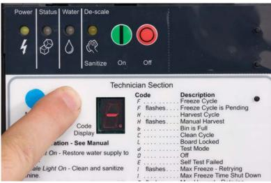
Put the control into the standby mode, then push and Hold the Clean button for 3 seconds. A "-" will be displayed. The pump and purge valve will be On for 30 seconds, repeat as needed to drain the reservoir.
