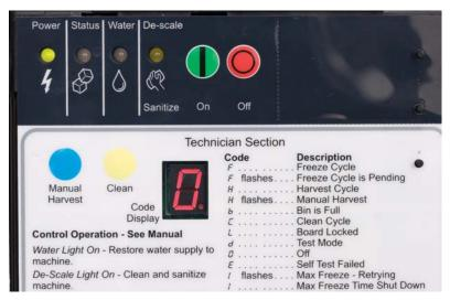
When power is supplied, the four lights at the top and the display indicator will blink on and off one time. Then the Power light will be on and the  $\varrho$  displayed.
